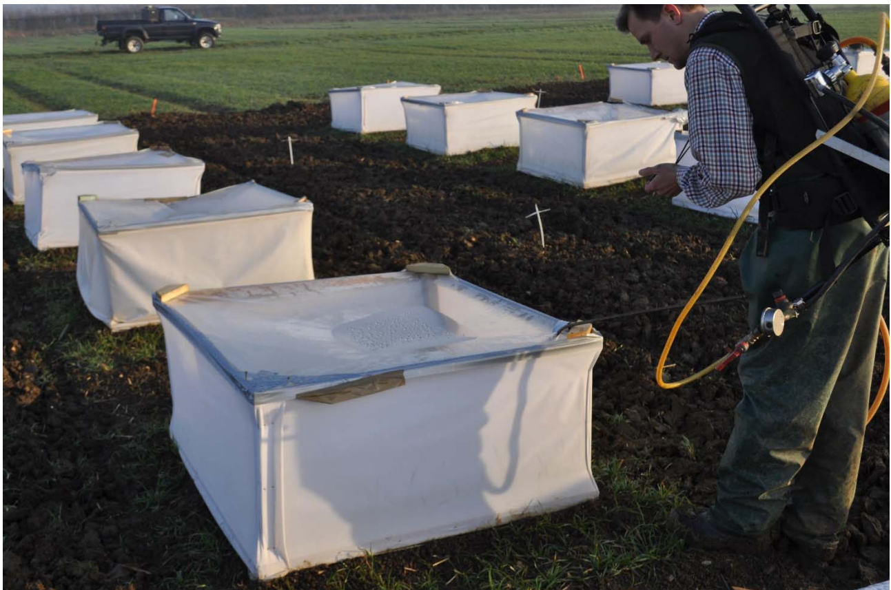
Figure 4. Wood-framed tents with breathable fabric sides and waterproof polyurethane top, ADAS Boxworth, February 2014. Small opening in top cover is used for inoculation with Z. tritici spores and for irrigation purposes. Frames in 2015 had additional cross-pieces under top cover to reduce rain water collecting on top.
